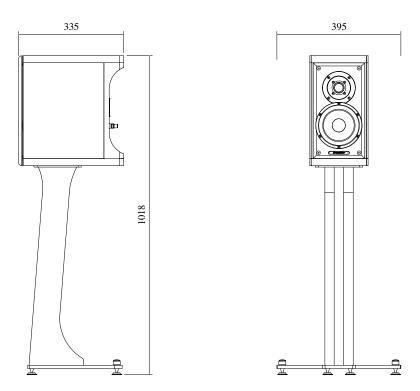
**SYSTEM:** 2 way vented box loudspeaker.
